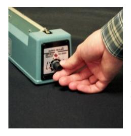
Plug power cord into 115V AC outlet and adjust timing dial to desired setting.
