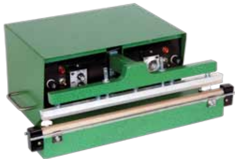
Automatic Sealer 18", 24" Seal Width Pressure Time 1-8 sec. Cycle Frequency 1-8 sec. Heat Seal Time 0.2 - 0.3 sec. Foot Pedal or Automatic Action
